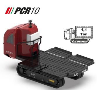
The PCR10 is a crawler vehicle without stabilisers and with a platform load capacity of 1.1T.
